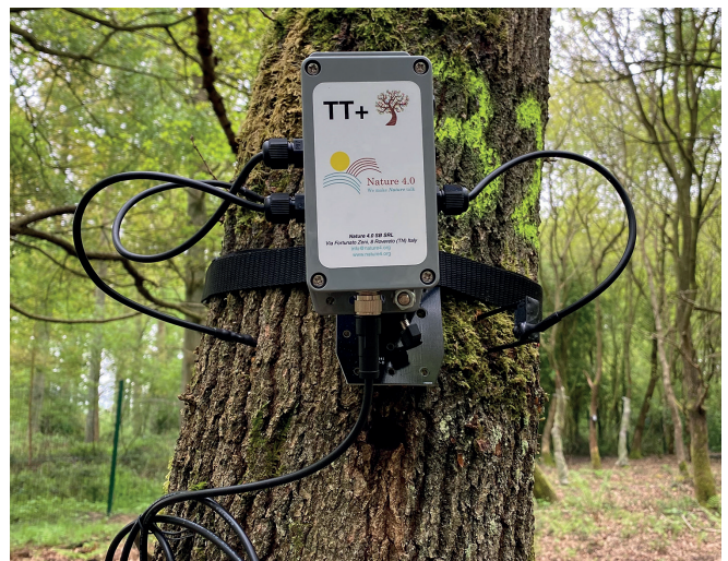
Figure 3: A TreeTalker mounted on the stem of an Oak tree at the field trial
